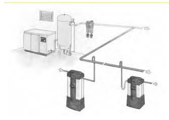
The Regenerative Desiccant Dryers will benefit users who have a specific need for Clean Dry Air (CDA) directly after a compressor, or for a particular application where the air is critical to the operating process or end product.
