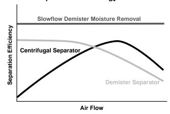
The oversized "slowflow" demister is non-velocity sensitive and therefore offers excellent liquid separation whatever the airflow.
