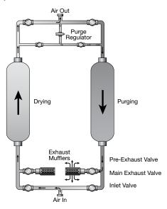
As the saturated compressed air flows up through the "on line" tower, its moisture content adheres to the surface of the desiccant. The dry compressed air is then discharged from the chamber into the distribution system.
