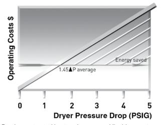
Poorly constructed heat exchangers and liquid separators create a high pressure differential across the dryer which leads to high operational costs and poor dewpoint performance.
