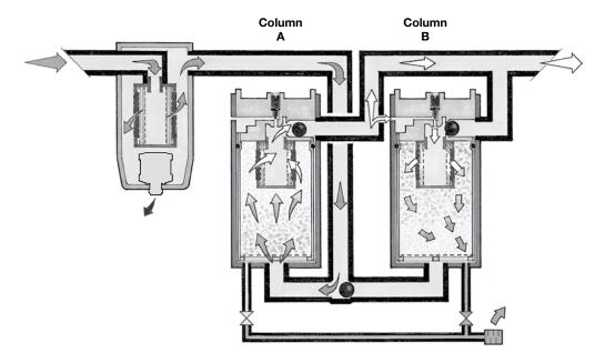
Prior to changeover, the right hand chamber (Column B) enters repressurisation where the exhaust.
